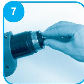
Push the sachet bung firmly into the end of the barrel.
