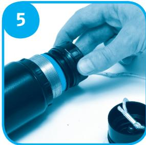
Insert the plunger into the rear end of the barrel.
